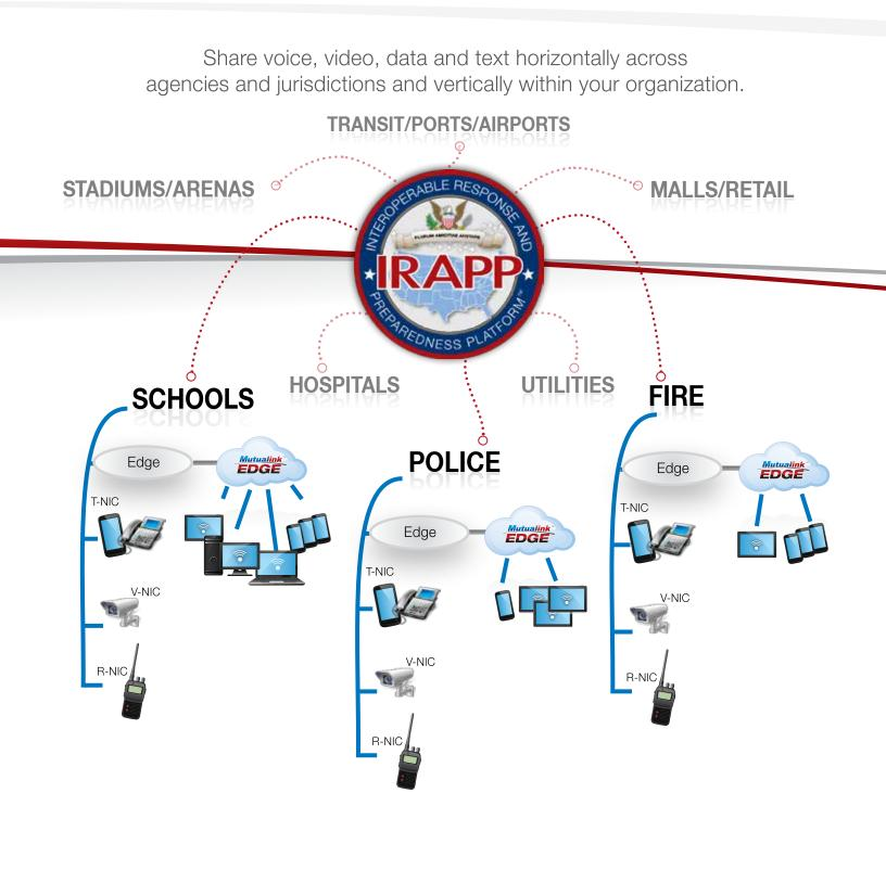
T-NIC: Telephone Network Interface Controller R-NIC: Radio Network Interface Controller V-NIC: Video Network Interface Controller
